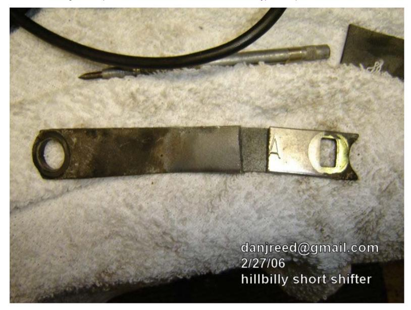
Take 1 stock shifter lever. And two chunks of metal, same thickness, about 1.5" long each
