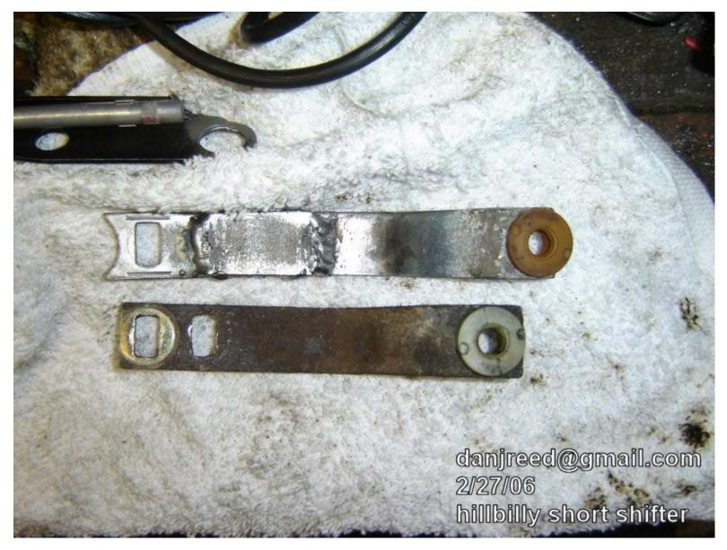
Weld the two plates to it about 1/2" or 5/8" longer or so...
